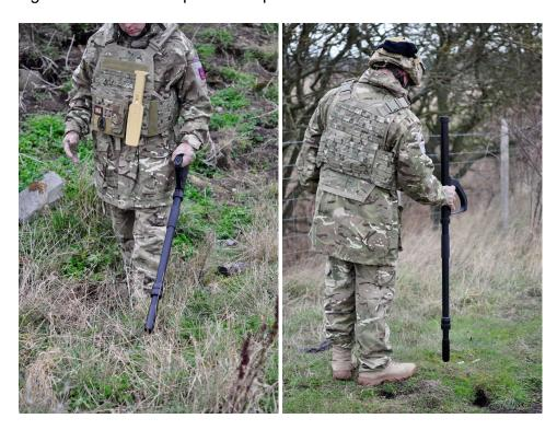
The detector is supplied in two parts that are easily assembled for use and split apart for transport using a simple hand-tightened collar fixing. Total time to make operational from packed transit case is less than 3 minutes. The detector uses sophisticated digital detection and performs automatic calibration to ensure that sensitivity is always optimal.
