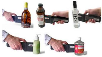
The system uses quasistatic electrical tomography to estimate the spatial distribution of the electric properties of a medium and determine the characteristics of a liquid regardless of the size of the container it is in, the thickness of the container's wall or any air gap between the device and the container. The electrical properties of the liquid (permittivity and conductivity) enable the system to unambiguously determine whether the liquid dangerous.
