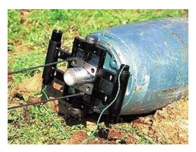
The **Rocket Wrench Defusing Device** can be deployed in either compact or increased diameter format. It can be used either clockwise or anti-clockwise without modification and is designed for quick and easy deployment. The wrench is powered by two electrically initiated 0.5 caliber power cartridges.
