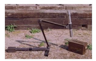
The equipment is operated by bespoke cartridges which are ballistically proven to offer consistent and effective performance. Cartridges are supplied in multiples of 10 packed in an H83 ammunition container complete with internal furniture, pistons and closure caps.
